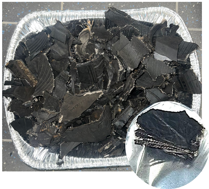
Rubber Aggregate (with Wire & Fiber) Avg Length = 5-7 cm < 1 wt% moisture
