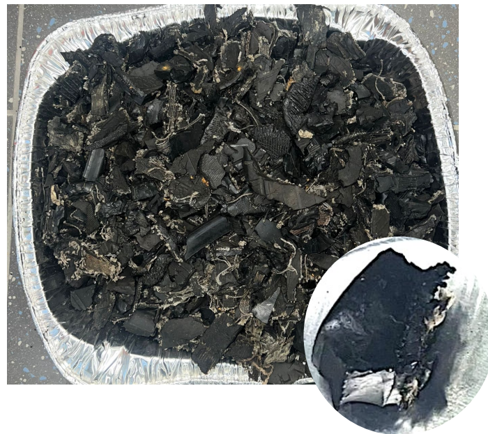
Rubber Mulch (with Fiber) Avg Length = 2-5 cm < 1 wt% moisture
