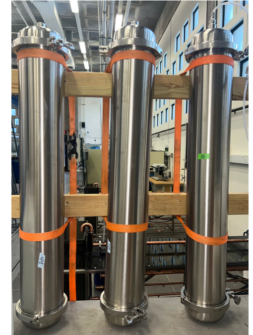
Three Percolation Columns in Parallel
