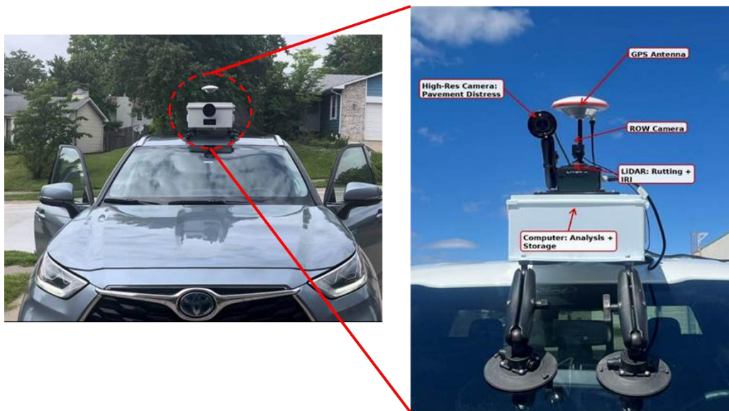
Figure 2. Portable Vehicle-Mounted Pavement Data Collection System
